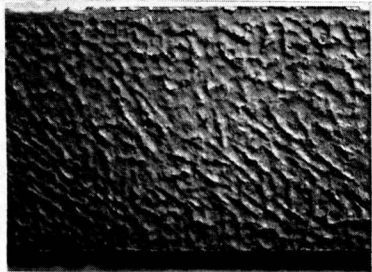
Fig. 8. Surface roughening of the 20Mo55Fe25Ni alloy during oxidation at 910°C. Top, surface roughening as a function of time ( 1\times before reduction for publication); bottom, surface after 224 min. ( 5\times before reduction for publication.)
