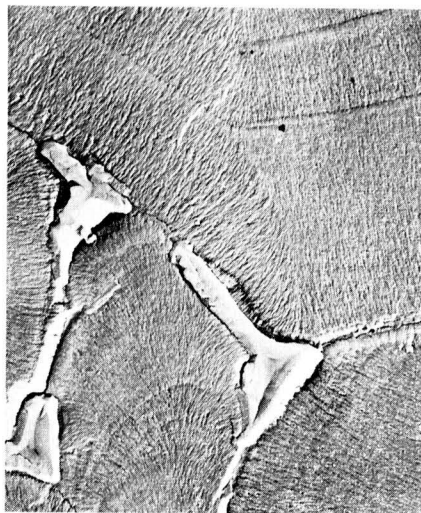
Fig. 9. Intersections of crystalline areas on a specimen almost completely crystallized. 5000X.
