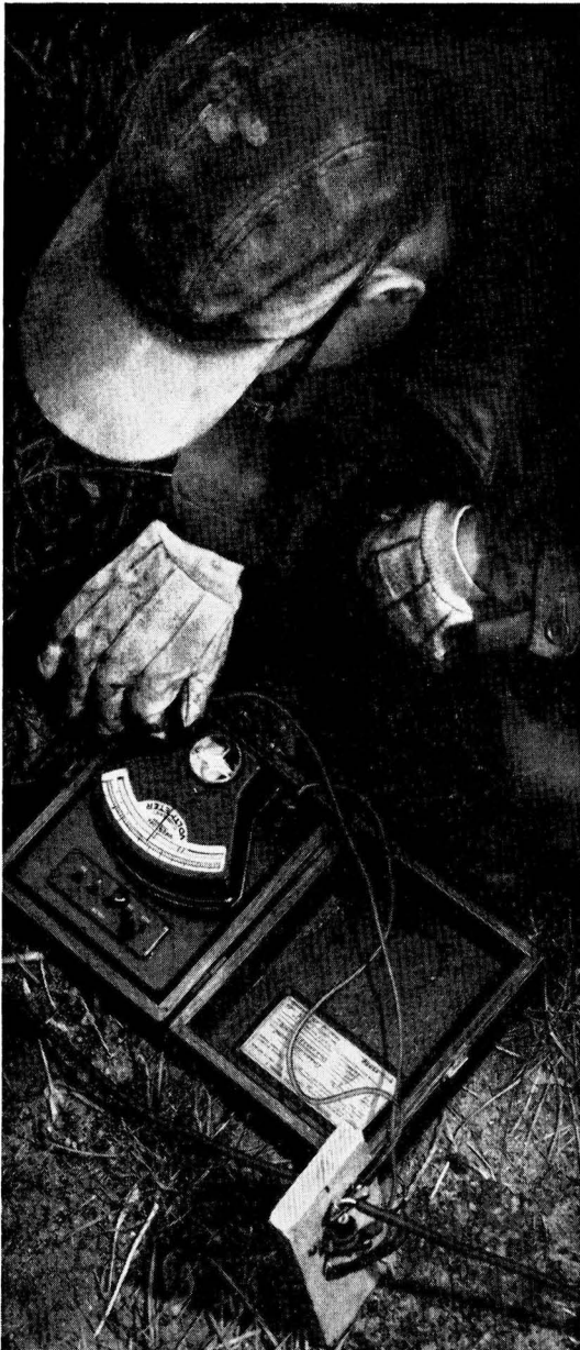
Field tests, made in various soils, have substantiated laboratory tests showing GALVOMAG does produce 20-30% more current than conventional anodes.
