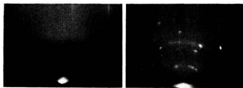
FIG. 4. (left) Pattern of cupric phosphate from water-washed specimen after heating to 450°C in vacuo.
