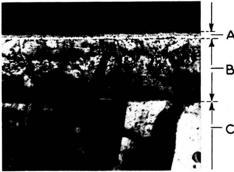
FIG. 4. Structure of a coating and diffusion layer produced on ingot iron (sample No. 14, Table II). A—Ti coating, B—diffusion layer, C—Fe core. Magnification 200X.
