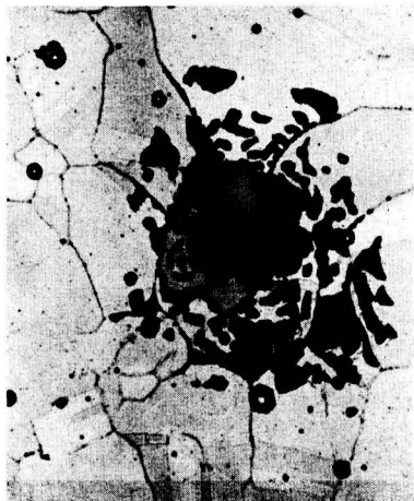
FIG. 11. Electrolytically formed pit. Mechanically polished AISI 304 steel (annealed) pitted electrolytically in 0.1N NaCl and then electrolytically etched in nitric acid to bring out grain boundaries. 350X before reduction for publication.
