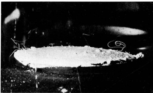
Fig. 4b. Stages in the growth of Cu filaments: after electrolysis for 27 hr.
