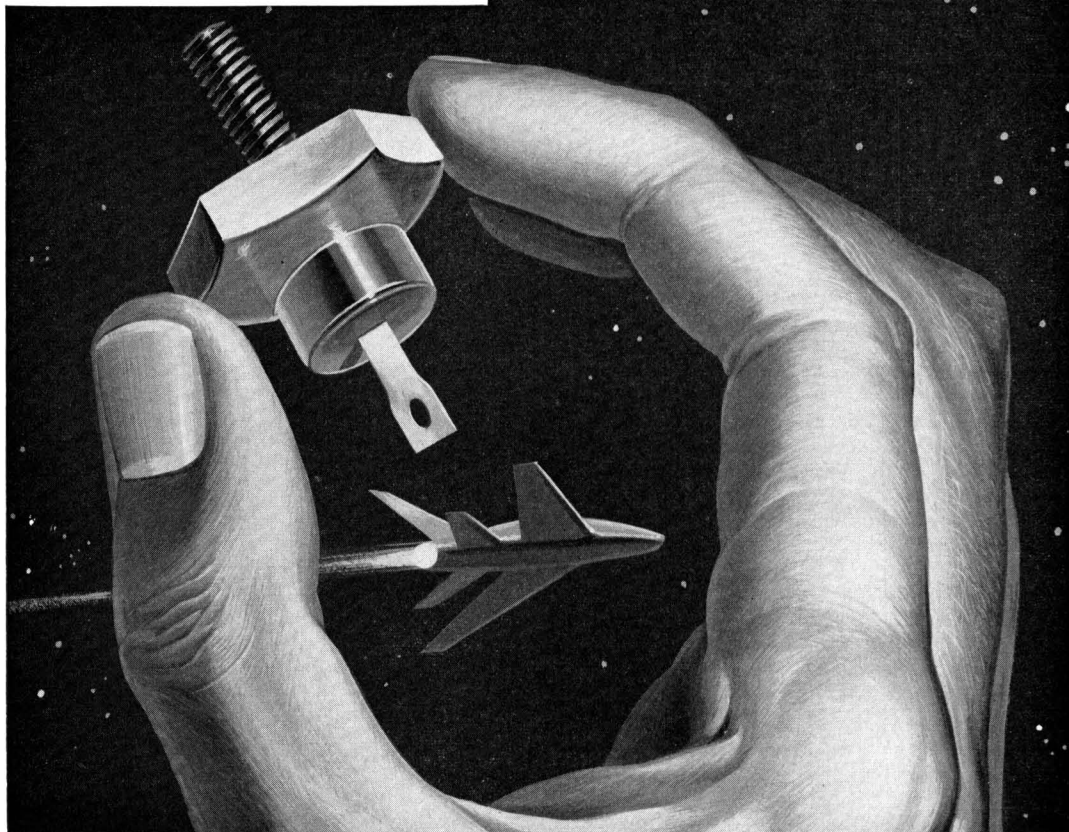
SILICON RECTIFIERS are finding increasing use at elevated temperatures in aircraft and missile applications by providing more power per pound.
