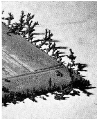
TYPICAL TREEING that occurs when using ordinary electrolytic tough pitch copper anodes.
