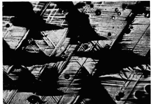
Fig. 5. Surface nitride (dark material) and distortion resulting from nitride precipitation on the (100) planes on a single crystal of Ta after 24 hr at 750°C in N<sub>2</sub> atmosphere. Magnification 500X before reduction for publication.
