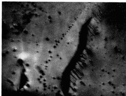
Fig. 7. Fractograph showing sites of nucleation of oxygen metal reaction on a grain surface. 500X before reduction for publication.
