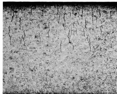
Fig. 7. Sheared edge of bent, stress-relieved specimen after 8-min exposure to 42% MgCl 2 . Electrolytic etch, 50X.
