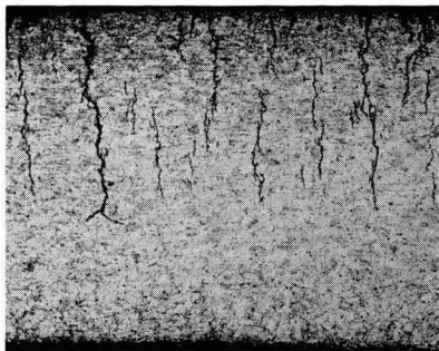
Fig. 10. Sheared edge of bent, stress-relieved specimen after 2-hr exposure to 42% MgCl_2 . Electrolytic etch, 50X.
