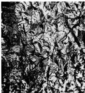
Fig. 21. Annealed at 600°C, after stressing (1000X)
