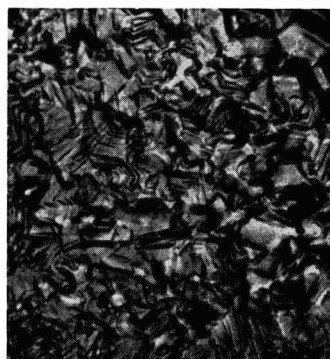
Fig. 19. Annealed at 600°C, before stressing (1000X)
