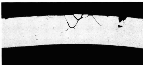
Fig. 13. Stressed Al-4% Cu binary alloy after exposure to 53 g/l NaCl with 12 ma anodic current for 4\frac{1}{2} min.
