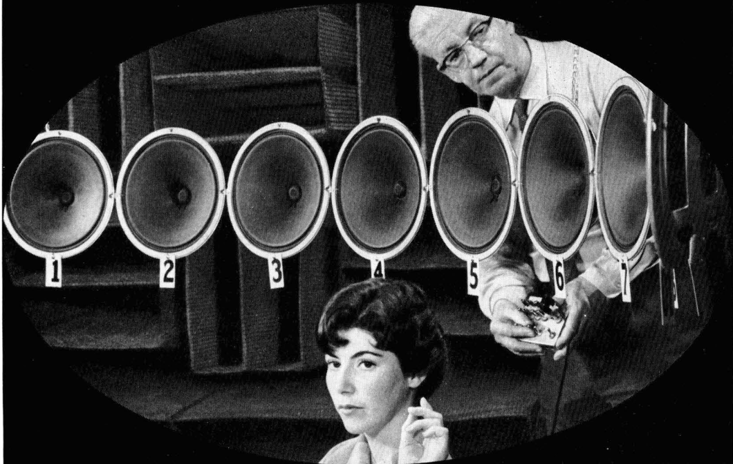
Which speaker is making the sound? In echoless chamber at Bell Labs, Robert Hanson measures test subject's ability to localize sounds—observes how two ears operate in partnership. This and other tests may point the way to better telephone instruments.
