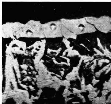
Fig. 5. Micrograph of a section from a sample plated with Ti in a KI-KF bath (Expt. 15, Table I). The microindentations in the Ti deposit correspond to a hardness of about 180 Vickers which is of high order and possibly results from some diffusion of the steel constituents into the Ti coating at the temperature at which the cathode was held during the electrolysis (950°C).
