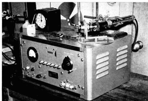
Fig. 2. Apparatus used for scanning the radioactivity on copper single crystal spheres having adsorbed thiourea- S^{35} .
