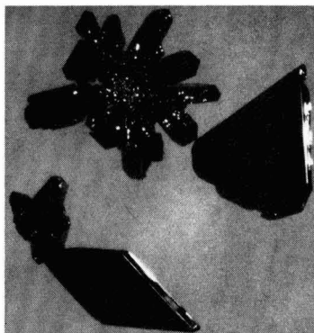
Fig. 1. InP crystals grown by reaction 8. Magnification 27X.
