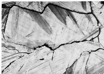
Fig. 9. L-170BC-gamma quenched and aged 475°C, 3 min (overaged), Ames etch, VHN-563, 30 kg.
