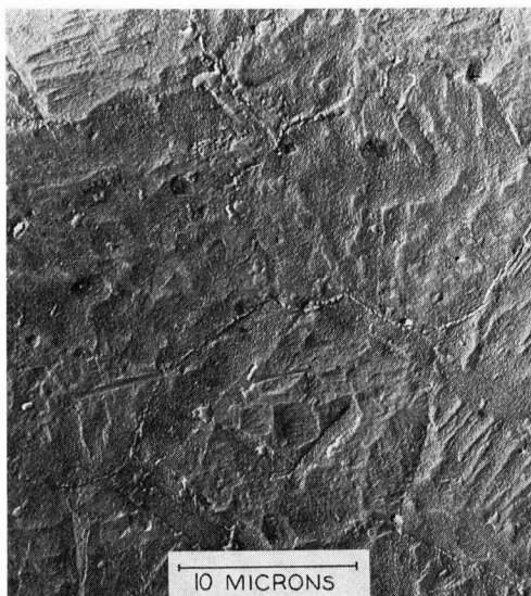
Fig. 5. Electron micrograph of 120Å thick nickel film. Magnification 7200X before reproduction.
