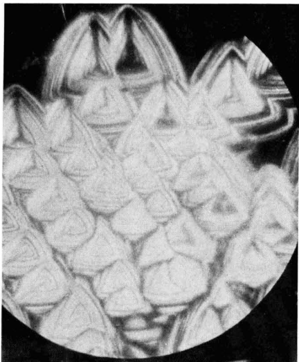
Fig. 2. One side of a GaAs ribbon after etching in \text{HNO}_3:\text{H}_2\text{O} (1:2). Magnification 500X before reduction for publication.
