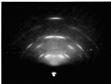
Fig. (A). A reflection electron diffraction pattern showing h.c.p. (10\bar{1}0) + f.c.c. (211) orientations for electrodeposited nickel (sulfate chloride bath, pH 5.1, c.d. 10 ma/cm 2 , bath temperature 25°C).
