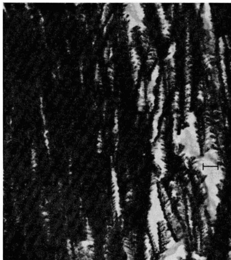
Fig. 3. Electron micrograph of the iron fibers as formed in the gel at 0.017 \text{ amp/cm}^2 . The electrolyte interface was at the top. 1000\text{\AA} scale marker.
