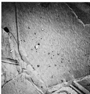
Fig. 8a. Electron micrographs of electrodeposited copper surfaces. See Table III for experimental details.
