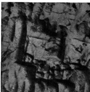
Fig. 9. Electron micrograph of {311} surface of copper oxidized in water in equilibrium with a helium-1% oxygen atmosphere for 18 hr. Direct carbon replica, preshadowed with palladium. 40,000X
