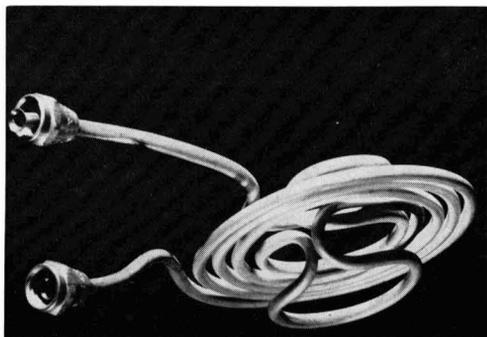
Fig. 1. Modified rf work coil
