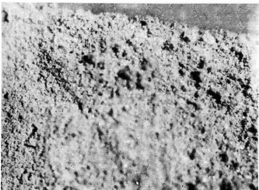
Fig. 2. Fine grained GaP underlying the surface mat of GaP needles. Magnification about 30X.
