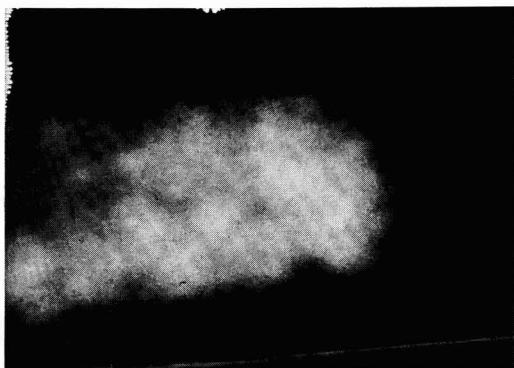
Fig. 7. GaP powder layer photographed under its own emission while d.c. excited.
