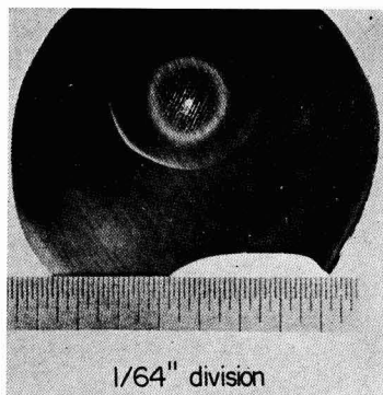
Fig. 3. Appearance of the Ge surface around the area facing the cathode.
