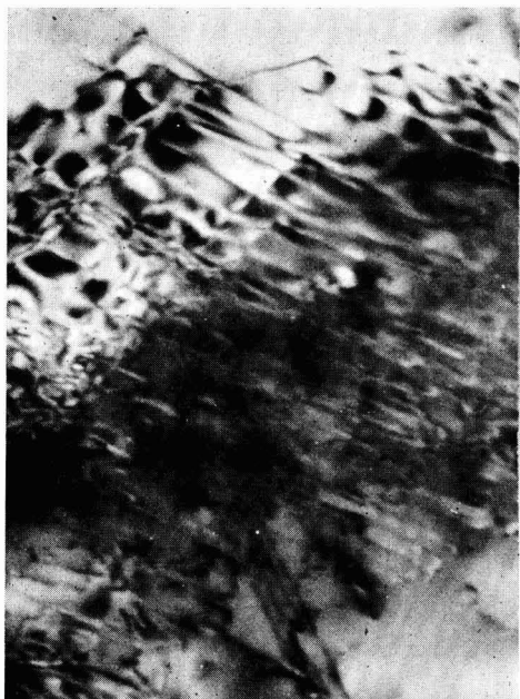
Fig. 2. Silicon abraded with No. 400 SiC paper. Severely strained dislocation network is present. Transmission electron micrograph 100,000X.
