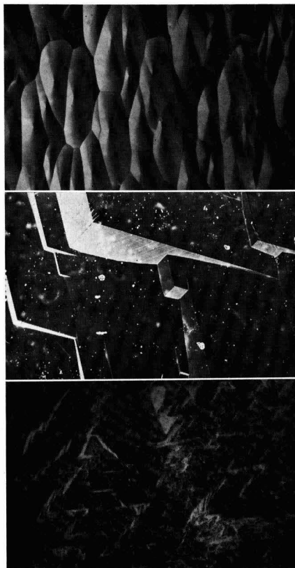
Fig. 7. Photographic views of epitaxial growth on a (top), (100); b (center), (111); and c (bottom), (113) planes. Magnification 45x.
