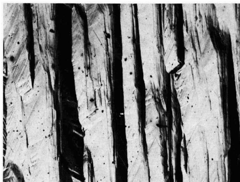
Fig. 1. Oriented growth on a (111) germanium surface after 16 hr at 885^{\circ}\text{C} . Magnification approximately 40x.
