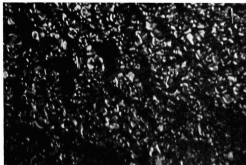
Fig. 3. Polycrystalline silicon film annealed 30 min at about 5°-10°C below the melting point of silicon. Magnification 520X.
