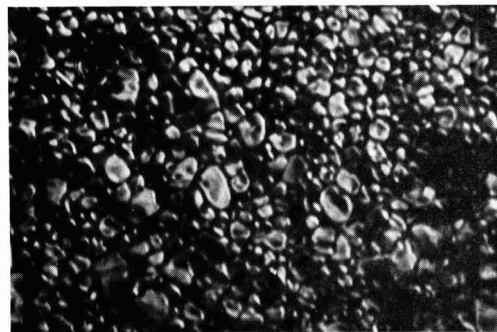
Fig. 4. Same as Fig. 3. except the annealing temperature was very close to, or at, the incipient fusion point. Magnification 520X.
