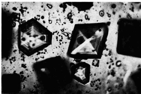
Fig. 4. As_2O_3 crystals on GaAs. Steps are discernible on the planes; etchant: aqua regia. Magnification 580X.
