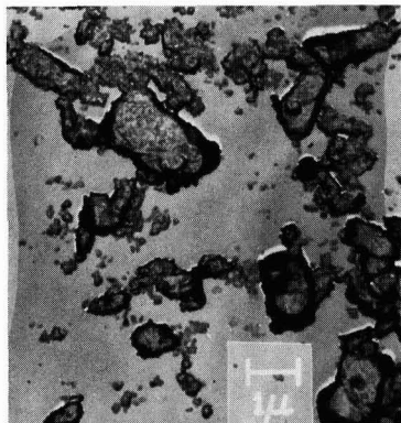
Fig. 10. \text{PbO}_2 obtained by extraction of \text{Pb}_3\text{O}_4 . The smallest individuals appear to be spheroidal, and the large particles may be conglomerates of these small units. There appears to be no tendency toward prismatic development.
