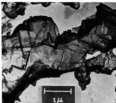
Fig. 6. Positive active material from a lead antimony cell. Massive prismatic conglomerates were characteristic of the active material in this sample.
