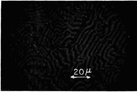
Fig. 4. Interference micrograph showing growth steps on the \{111\} plane where faults propagating in the three inclined \{111\} planes reach the surface.
