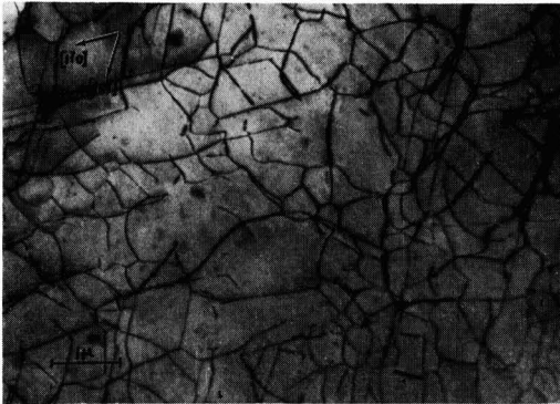
Fig. 7. Low-magnification micrograph reveals traces of dislocations lying in the three \{111\} planes, projected upon the plane of observation. In this micrograph (taken at a depth of 1/3\mu ), an unusually high dislocation density (for this depth) is found, not characteristic for this level when compared to many other observations.
