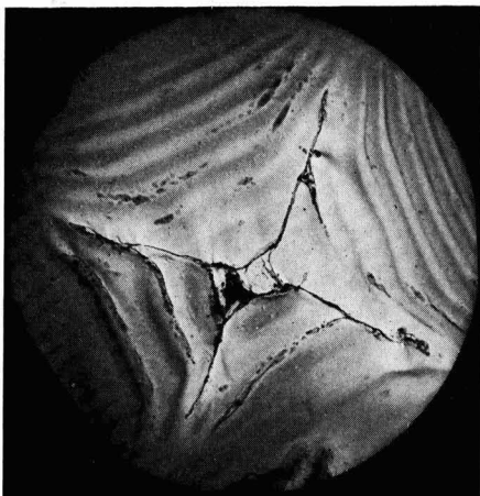
Fig. 2. Carbon replica of stepped pyramid on (100) tungsten surface. Magnification 1500X.
