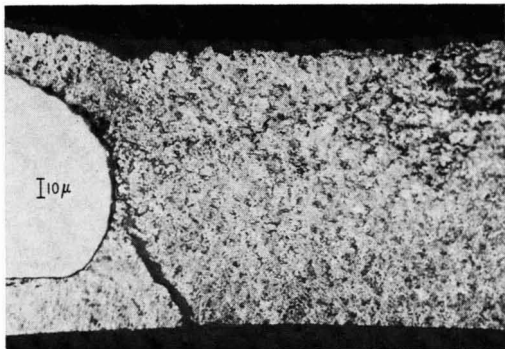
Fig. 2. Photomicrograph of a sectioned electrode showing the surface film on one side. Electrode No. 375. Body: 34 mg Pt black, 3.1 mg Teflon/cm 2 ; film: 2.4 mg Teflon/cm 2 ; nickel screen, 40 mesh; 4.5 mil wire. Magnification approximately 330X.
