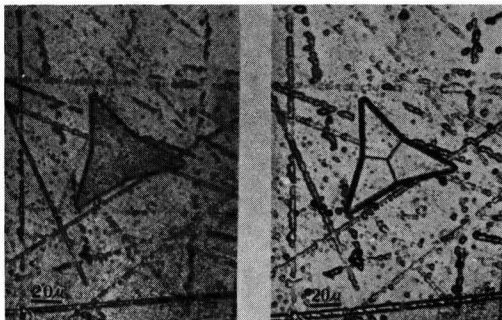
Fig. 3. Etch figure of tripyramids: (a) (left) etched with Sailer etch for 1 hr after partial removing of the hillock; (b) (right) the same samples were etched successively with iodine etch for 10 sec.
