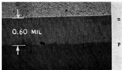
Fig. 3. Effect of Cu diffusion on the formation of the \text{SiO}_4^+ donor level in 54 ohm-cm p-type Si; beveled X-section depth magnified 10X; microscope 60X. (a) Typical n-layer formed by diffused oxygen.
