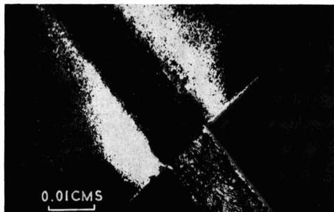
Fig. 1. Polycrystalline germanium film and aluminum alloy zone on sapphire substrate after heating for 8 hr in a temperature gradient of  $150^\circ\text{C}/\text{cm}$ .
