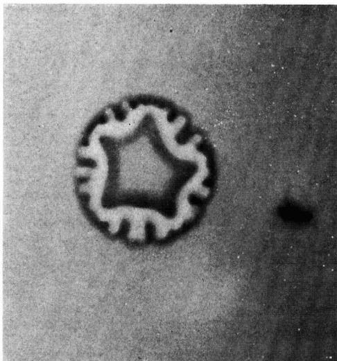
Fig. 4. Rosettes were formed on 500Å-thick palladium evaporated on an iron crucible which was hydrogen charged from the inside. Magnification 700X.
