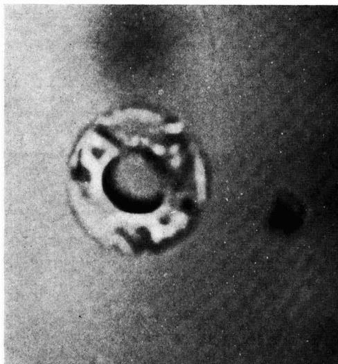
Fig. 5. Rosette shown in Fig. 4 deformed after a few hours. Magnification 700X.
