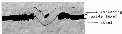
Fig. 9. Section of an AISI 304 sample marked with a diamond point and oxidized for 1000 hr in steam at 500°C.
