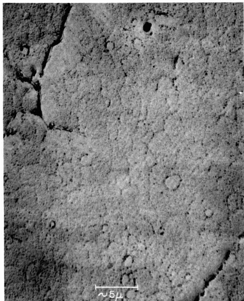
Fig. 8. Oxide formed with H_2O , electron micrograph. Magnification ca. 6700X.
