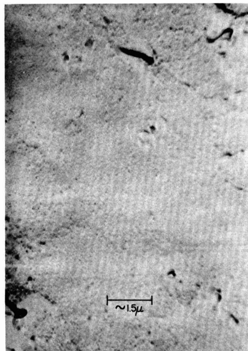
Fig. 5. Thermal oxide, electron micrograph replica. Magnification ca. 23,330X.
