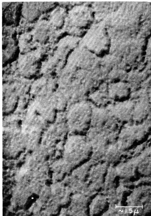
Fig. 4. Chemical oxide, electron micrograph, replica. Magnification ca. 23,330X.
