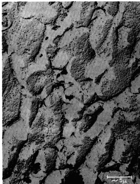
Fig. 7. Oxide formed with \text{H}_2\text{O}_2 , electron micrograph. Magnification ca. 6700X.
