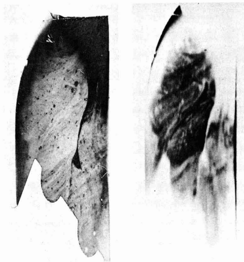
Fig. 6(a). (left). (400) topograph reveals inhomogeneous regions in the (100) deposit of (Ga,In)As; the alloy reflection was used to form the topographic image: (b) (right) the relative contrast was reversed when the GaAs diffraction angle was employed to obtain the (400) topograph.
