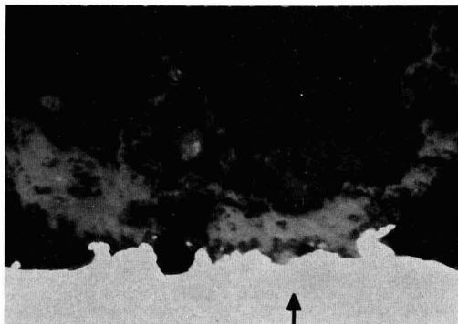
Fig. 3. Cross section of scale formed on Fe-18.0% Cr by 1-hr oxidation. Magnification 1000X.
