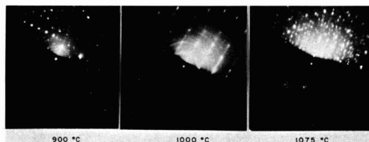
Fig. 3. Electron diffraction patterns of molybdenum deposited on (111) silicon substrate.
