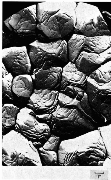
Fig. 7. Electronmicrograph of a Ge (100) surface oxidized for 2 hr in 15.6N HNO 3 at 27.5°C. The oxide layer is seen to be composed of densely packed crystalline oxide nuclei.
