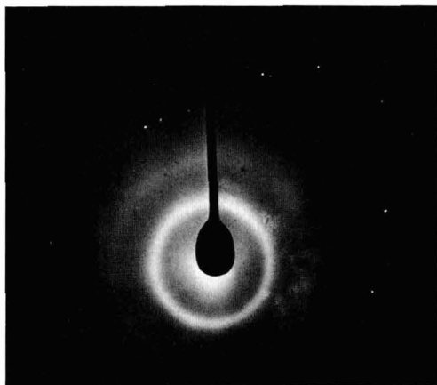
Fig. 8. Typical diffraction pattern of as-deposited Ni-P islands, and fresh thin Ni-P films (P content of 5 w/o).
