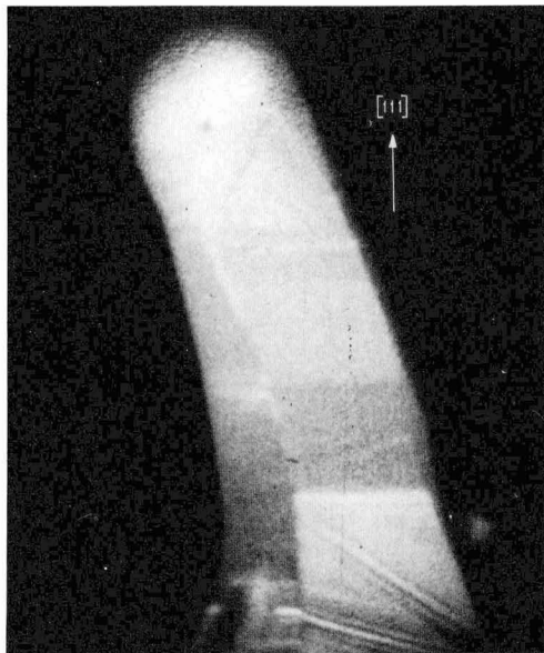
Fig. 6. Curved silicon crystal photographed during nonisothermal growth. Magnification approximately 50X.
