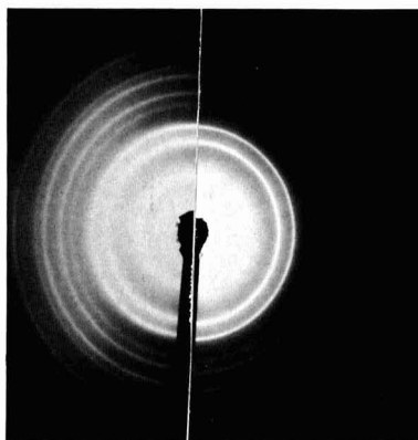
Fig. 3. Transmission electron diffraction patterns produced by evaporated gallium arsenide films. A(left), calcium fluoride substrate; B(right), sodium chloride substrate.
