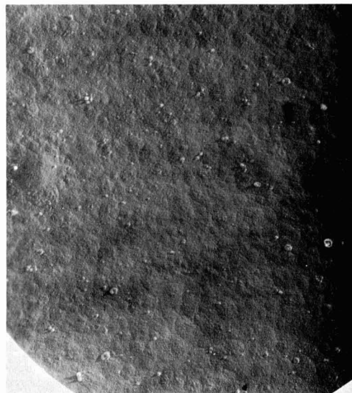
Fig. 4. Electron micrograph of a V_2O_5 film on sapphire at ca. 7600\times .
