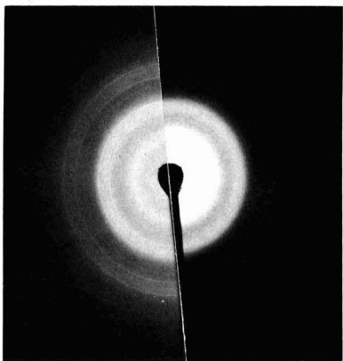
Fig. 2. Transmission electron diffraction patterns produced by evaporated germanium films. A(left), laser evaporation; B(right), conventional evaporation.
