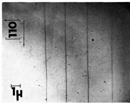
Fig. 4. SOT x-ray topograph of diffused structures similar to Fig. 3 with the following thicknesses of surface removed: a, nothing removed; b, 0.5\mu ; c, 10.0\mu ; d, 19.0\mu .
