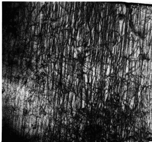
Fig. 4. X-ray topograph of a gallium antimonide wafer exhibiting a high density of dislocations. Two sets of dislocations can be observed. One set of rather long dislocations appears aligned along the \langle 111 \rangle growth direction, the other consists of a network of dislocation loops. Ag, K\alpha radiation (220) reflection. Magnification ca. 40X.
