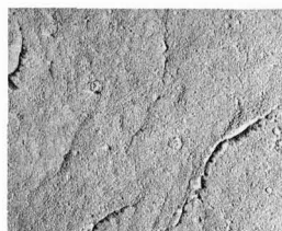
Fig. 3. Typical surface replica of martensitic specimen oxidized to the range of linear kinetics. Oxygen uptake: 1.56 mgO/cm 2 . 14,665X.
