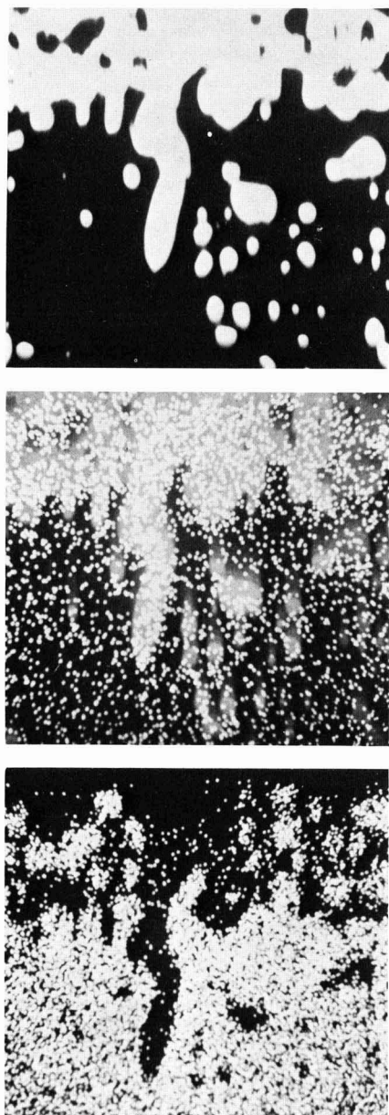
Fig. 3. Electron probe images of sample in the two-phase field spinel + alloy, 1000X. (a) Upper micrograph—electron backscatter image. The spinel phase appears as bright and the alloy phase appears as dark. (b) Middle micrograph—Fe- K_{\alpha} x-ray image showing distribution of iron in the two phases. (c) Lower micrograph—Ni- K_{\alpha} x-ray image showing nickel distribution.
