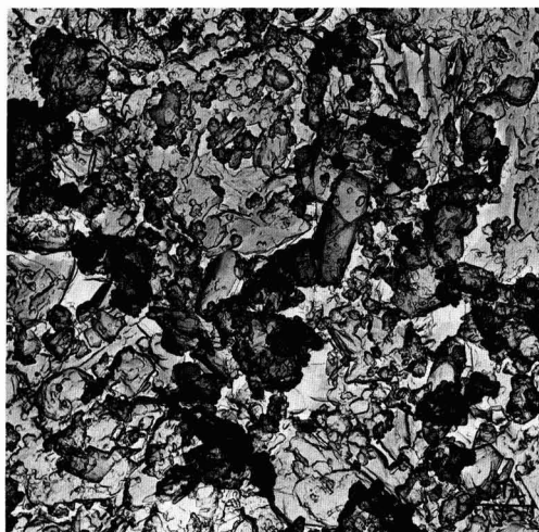
Fig. 6. Interior active material of a 1-hr formed electrode. Compounds present are 3\text{PbO} \cdot \text{PbSO}_4 \cdot \text{H}_2\text{O} , \text{PbSO}_4 , orthorhombic and tetragonal-PbO, and free Pb.
