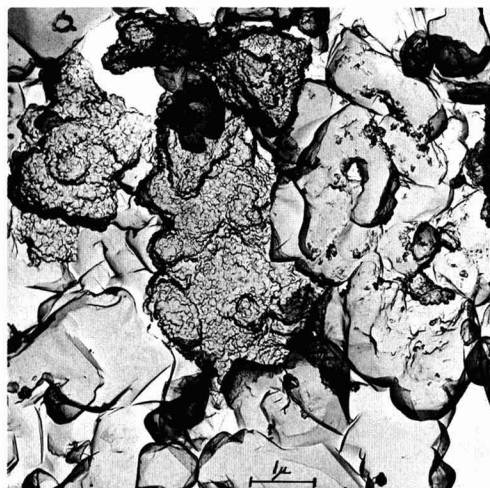
Fig. 8. Interior of positive electrode after 11 hr of formation showing large \text{PbSO}_4 crystals being converted to crystalline aggregates of \beta\text{-PbO}_2 .
