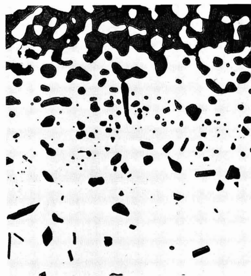
Fig. 1. Equilibrium two-phase fields wustite-alloy and the spinel-alloy. In both micrographs, the dark phases are the oxide phases and the bright phase is the alloy phase: (a) upper micrograph—wustite + alloy etched in 5% HCl in ethyl alcohol, 250X; (b) lower micrograph—spinel + alloy etched in 50% HCl in water, 320X.
