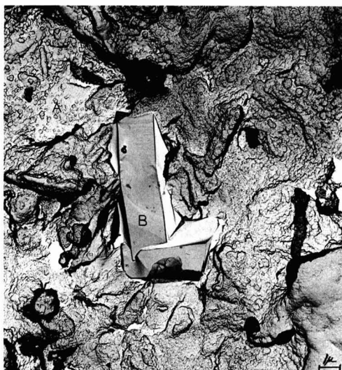
Fig. 10. Interior of active material after 15 hr of formation showing undeveloped crystalline masses (A) and large well-developed crystals believed to be \alpha\text{-PbO}_2 (B). Active material area is very near a grid member. These and similar areas were observed in both 15- and 20-hr formed electrodes.
