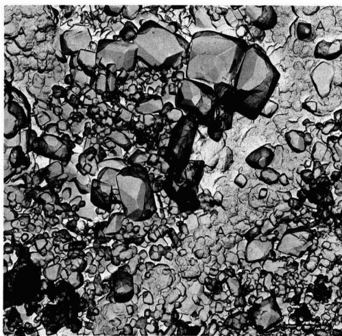
Fig. 3. Electrode surface after 5 hr of formation: (a, top) active material next to a grid member; small crystals are \beta -PbO 2 ; (b, bottom) active material further away from a grid member. Well developed crystals are PbSO 4 . The initial appearance of \beta -PbO 2 occurs as rounded crystal agglomerates and appear in areas A of the electron micrograph.
