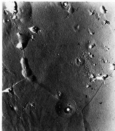
Fig. 8. Minor flaws produced by cracking of anodic oxide around intermetallic particles in a Zircaloy-2 specimen anodized in ammonium borate (Specimen Bh 306, 18 V). X 5000.
