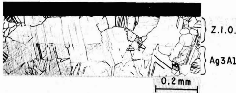
Fig. 5. Cross-section micrograph showing a zone of internal oxidation (Z.I.O.) in a Ag3Al sample which was oxidized for 29 ksec at 823°K. Etched.
