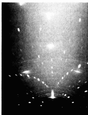
Fig. 2. X-ray photograph of precipitates and matrix. Note the spotty curved lines of polycrystalline \beta\text{-Ga}_2\text{O}_3 superimposed on the monocrystalline GaP pattern.
