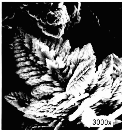
Fig. 1. Electroplated dendrites from saturated solution of potassium zincate (100 mA/cm 2 ).
