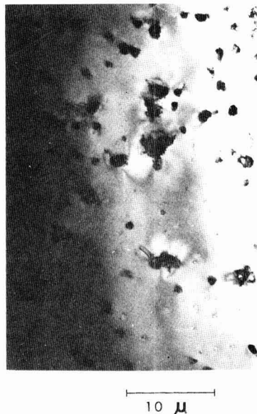
Fig. 2. A micrograph of the GaAs layer within 1 \sim 2\mu from the interface, obtained by using a transmission electron microscope. A high density ( 10^5 \sim 10^6 cm -2 ) of precipitates probably due to alloying are shown to exist. Prior to measurements, the Ge substrate was completely removed from the GaAs layer by chemical etching with hot H_2O_2 solution (5).
