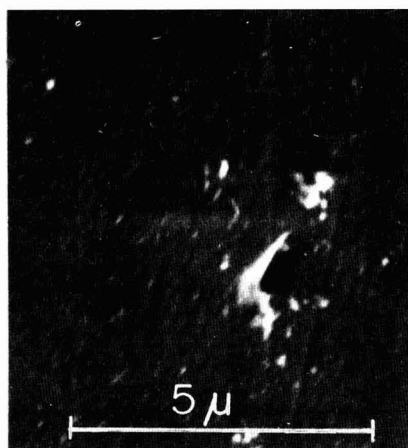
Fig. 8. Scanning electron micrographs with different magnifications of film formed by anodizing Be in electrolyte A for 1.5 min with a preset current of 3 mA/cm 2 and a preset potential of 50V. The films are significantly free from porosity.
