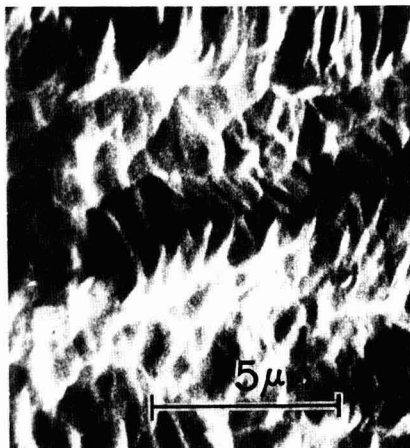
Fig. 3. Scanning electron micrographs with different magnifications of film formed by anodizing Be in CrO 3 -HNO 3 for 2 min at 30 mA/cm 2 . The films are markedly porous, the scale of the porosity being 100-1000 nm.
