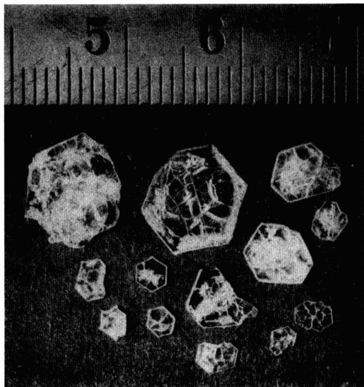
Fig. 1. Crystals of \text{Na}_2\text{O} \cdot 7.43\text{Ga}_2\text{O}_3 grown from a NaF flux
