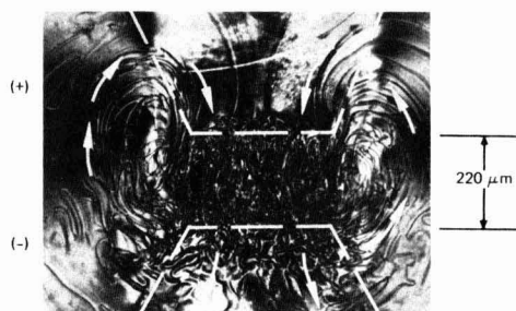
Fig. 7. Flow pattern of LC in a type B cell. Alignment of LC was perpendicular to the surface of the glass substrate. Photographs were taken with crossed polarizers. Dopant: 0.2% DBF. Applied voltage: 120V.
