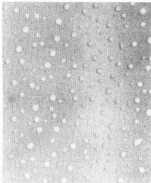
Fig. 6. Photograph of a silica film with bubbles trapped in the film. If these bubbles remain in the film when it is drying, the damage shown in Fig. 3 results. (Magnification 100X.)
