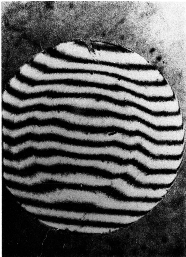
Fig. 7. Interferogram of C-1 glass cathode after 135 mC. This is the face toward the discharge.
