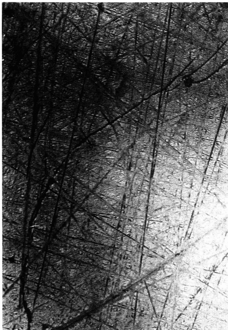
Fig. 11. Photomicrograph of a C-1 glass anode, side in contact with stainless steel. A fracture traverses from the upper right to the left lower edge. The smaller dimension of the figure is 1 mm of the plate.
