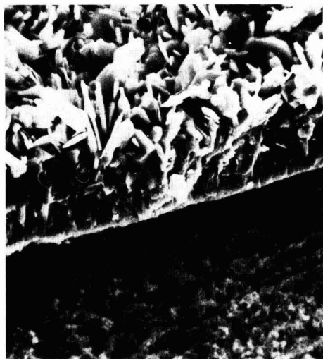
Fig. 3. Cross section of an alloy I specimen sulfidized at 850°C in 6.2 \times 10^{-2} Torr sulfur for 4 hr ( \times 1000 ).
