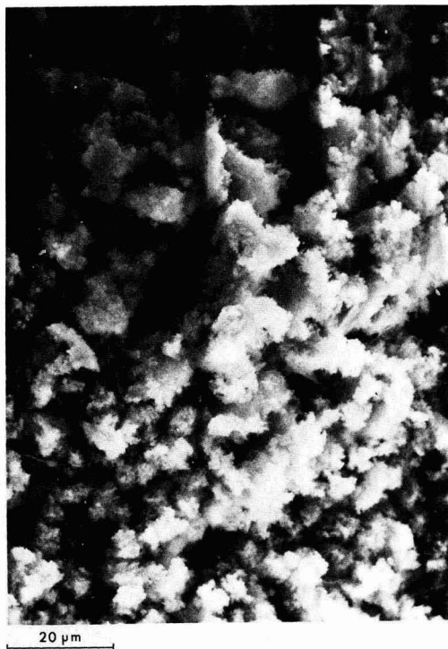
Fig. 11. SEM picture of Li surface after five days of storage in PC with 0.1% \text{H}_2\text{O} , 1000 \times .
