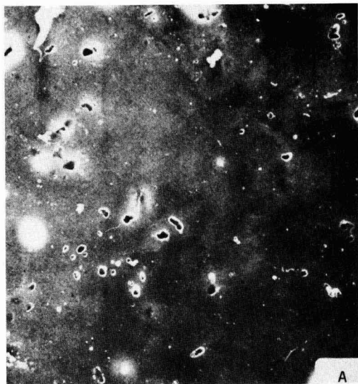
Fig. 5. Cross sectional image of 2024-T3 aluminum alloy specimen anodized in 170 g/l \text{H}_2\text{SO}_4 at 15°C and at alternating constant voltage of 26V for 30 min. EPMA observation.
