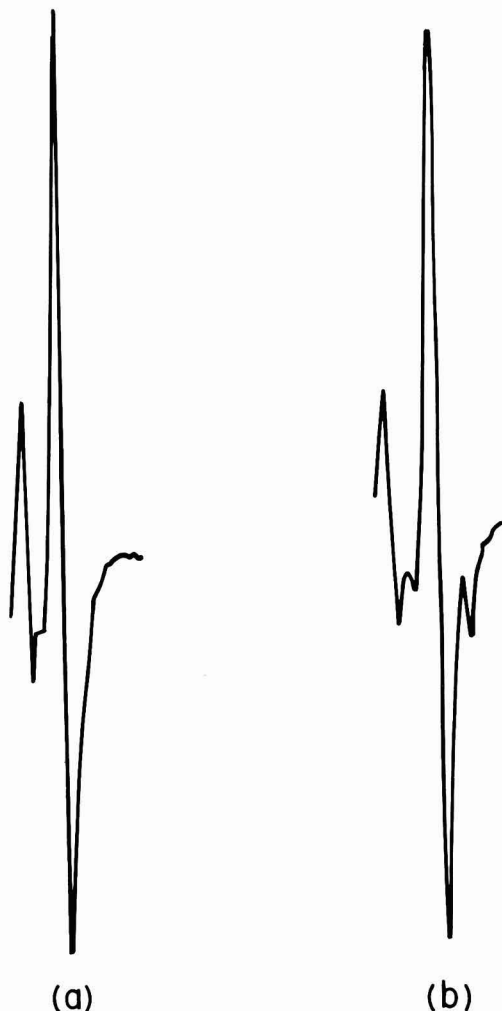
Fig. 2. N KLL Auger electron peaks from (a) specimen oxidized at 95°C and (b) NbN.
