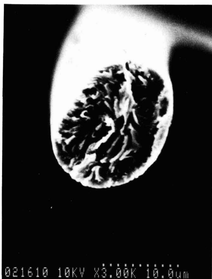
Fig. 1. SEM micrograph of cross section of the 3000°C treated mesophase-pitch-based carbon fiber.
