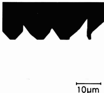
Fig. 3. Photomicrograph of a (110) cleaved plane of an overgrown layer for the 90° tungsten stripe direction which corresponds to \langle 110 \rangle .
