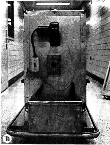
Fig. 1 Transportation unit: (1a) Complete unit with transfer cases in place; (1b) power supply, and (1c) transfer case and inner liner which holds 7 pigs. The blood seen on the inner liner is from umbilical bleeding which sometimes occurs during shipping because of the activity of the pigs crowded together.
