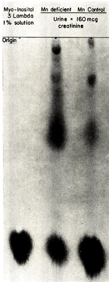
Fig. 2 Paper chromatogram with standard myoinositol (left) and urine preparations equivalent to 160 \mu g creatinine. Ethyl acetate-pyridine-water, 40:11:6. Running time 200 hours. Silver nitrate detection.
