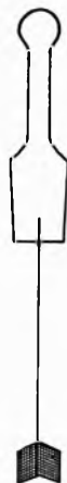
FIG. 1. Stopper with platinum wire and gauze attached as used in the flask combustion method.
