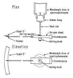
FIG. 1. Device for obtaining a magnified indication of the setting of the wavelength scale.
