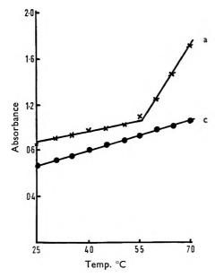
FIG. 1. Solubilisation of Waxoline Yellow IS.  $\times$ , 0.02M dodecylpyridinium bromide. •, 0.01M tetradecylpyridinium bromide.
