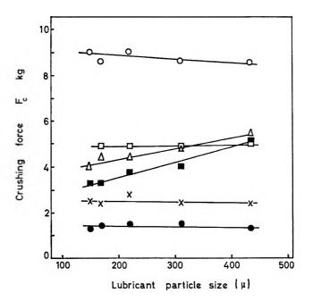
FIG. 7. Effect of lubricant particle size on crushing strength.
