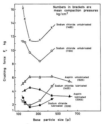
FIG. 3. Effect of base particle size on crushing strength.
