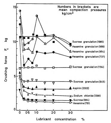
FIG. 6. Effect of lubricant concentration on crushing strength.
