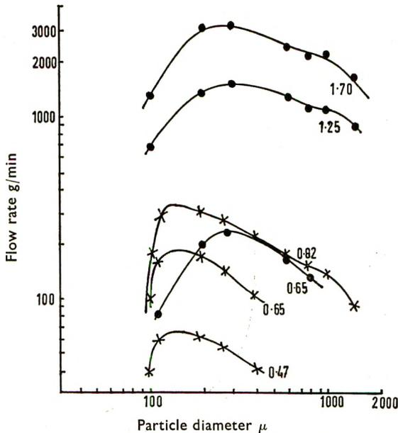
FIG. 6. Effect of orifice and particle diameter on rate of flow. ● = Magnesia. × = Lactose. Figures on the curves are the orifice diameters in cm.
