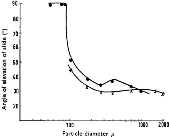
FIG. 4. Effect of particle diameter on angle of friction. ● = Magnesia. × = Lactose.
