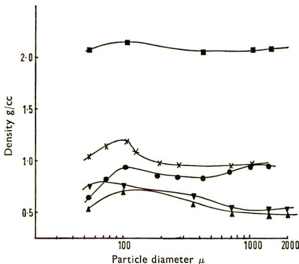
FIG. 3. Effect of particle diameter on powder density. ● = Bulk density of magnesia. × = Tap density of magnesia. ■ = Compacted density of magnesia at 160 kg/cm<sup>2</sup>. ▲ = Bulk density of lactose. ▼ = Tap density of lactose.
