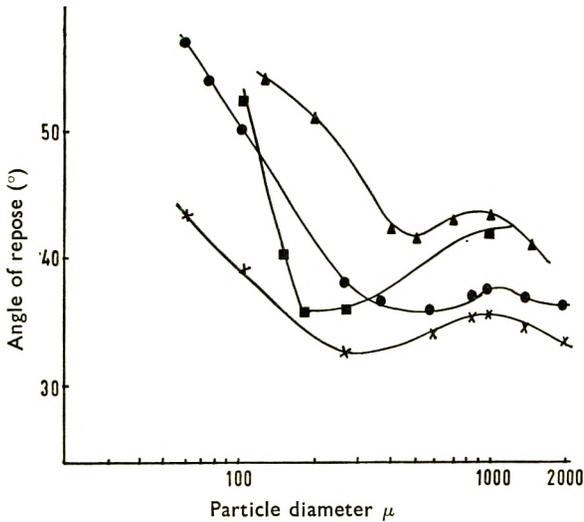
FIG. 5. Effect of particle diameter on angle of repose. ● = Magnesia. × = Lactose. ■ = Silica sand. ▲ = Sulphathiazole.
