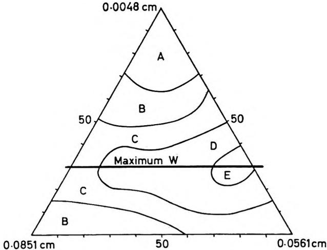
FIG. 4d. Flow contours for ternary system  $D_{Pc1} = 0.0561$  cm,  $D_{Pc2} = 0.0851$  cm,  $D_{P1} = 0.0048$  cm.  $D_o = 0.898$  cm. Flow rate (W g/min): A = <400, B = 400-500, C = 500-600, D = 600-640, E = >640.
