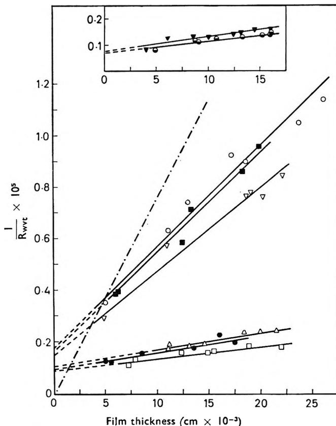
FIG. 3. Variation of the reciprocal of the water vapour transmission rate ( $R_{wvt}^{-1}$ ) with film thickness for the three film systems. Key: as in Fig. 1;  $\bullet$ — $\bullet$ , theoretical plot for Fickian system having permeability constant of  $0.013 \times 10^{-5}$ .
