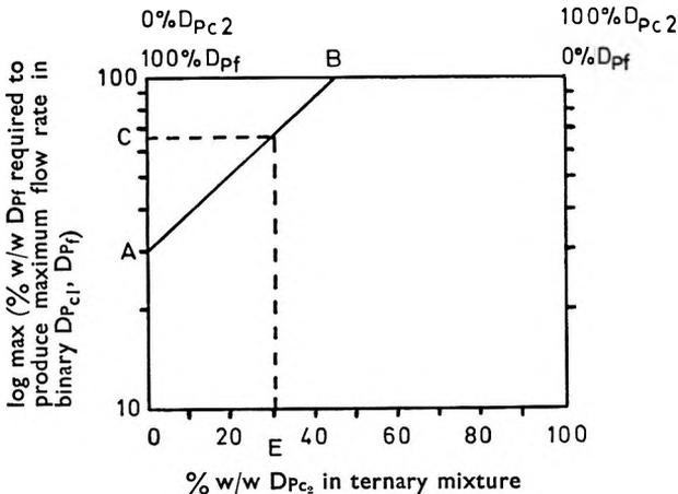
FIG. 5. Method for estimating composition for maximum flow rate in a ternary system. D<sub>Pc1</sub> = 0.0253 cm. D<sub>Pc2</sub> = 0.0561 cm. D<sub>Pf</sub> = 0.009 cm.
