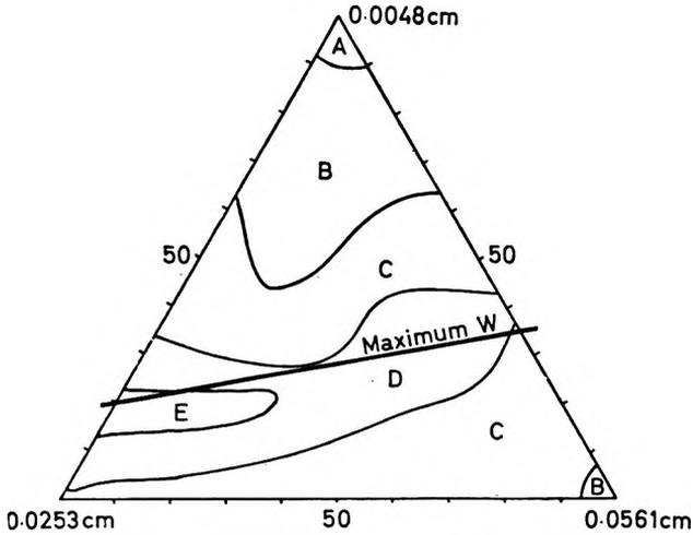
FIG. 4a. Flow contours for ternary system  $D_{Pc1} = 0.0561$  cm,  $D_{Pc2} = 0.0253$  cm,  $D_{Pr} = 0.0048$  cm.  $D_o = 0.74$  cm. Flow rate ( $W$  g/min): A =  $<200$ , B =  $200-300$ , C =  $300-400$ , D =  $400-420$ , E =  $>420$ .
