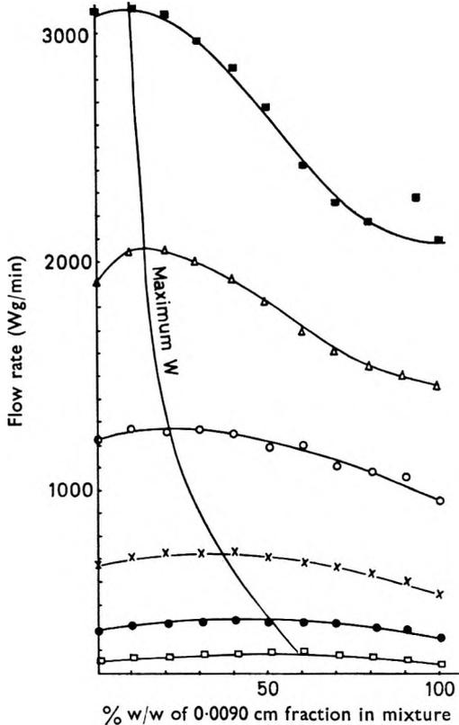
FIG. 3. Effect of orifice diameter on the flow rate of the binary mixture  $D_{r_c} = 0.0253$  cm,  $D_{r_f} = 0.0090$  cm.  $D_o$  in cm: ■ = 1.686, △ = 1.353, ○ = 1.140, × = 0.398, ● = 0.740, □ = 0.603.
