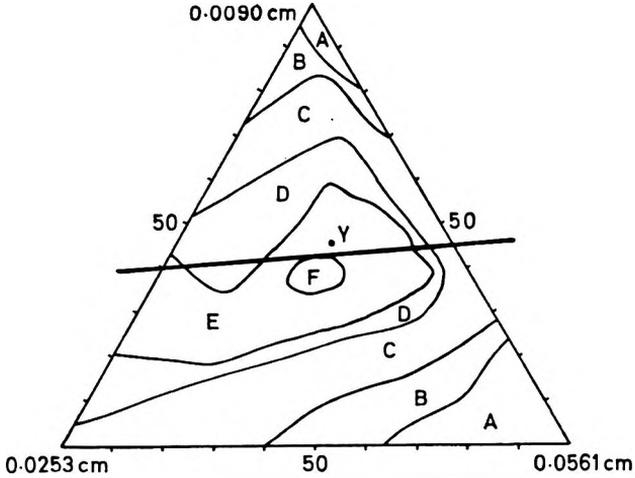
FIG. 4c. Flow contours for ternary system  $D_{Pc1} = 0.0561$  cm,  $D_{Pc2} = 0.0253$  cm,  $D_{P1} = 0.0090$  cm.  $D_o = 0.898$  cm. Flow rate (W g/min): A = <600, B = 600-650, C = 650-700, D = 700-720, E = 720-730, F = >730.
