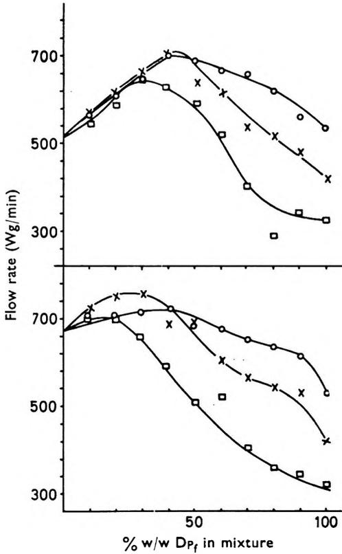
FIG. 2. The effect of particle size on flow rate of binary mixtures of coarse and fine components through a circular orifice  $D_o = 0.898$  cm.  $D_{p_c}$  in top graph =  $0.0561$  cm and in bottom graph =  $0.0253$  cm.  $D_{p_f} = 0.0048$  cm ( $\square$ ),  $0.0071$  cm ( $\times$ ) and  $0.0090$  cm ( $\circ$ ).
