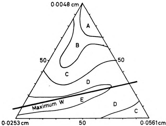
FIG. 4b. Flow contours for ternary system  $D_{Pc1} = 0.0561$  cm,  $D_{Pc2} = 0.0253$  cm,  $D_{Pr} = 0.0048$  cm.  $D_o = 0.898$  cm. Flow rate ( $W$  g/min): A =  $<400$ , B =  $400-500$ , C =  $500-600$ , D =  $600-700$ , E =  $>700$ .
