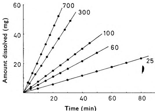
FIG. 1. The dissolution of aspirin at various stirring rates (rpm). Beaker method using compressed discs (diameter 1.3 cm) of aspirin (form I) in 0.1N HCl at 37°.
