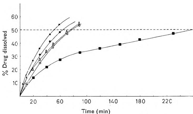
FIG. 3. *In vitro* dissolution of commercial aspirin tablets, P ▲, Q ●, R △, S ○, T ■. Beaker method at 62 rpm in 0.1N HCl at 37°.
